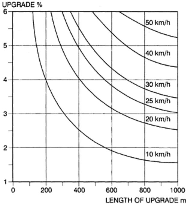
Figure 8.2 Speed reduction effect of upgrade (ref. 4).
