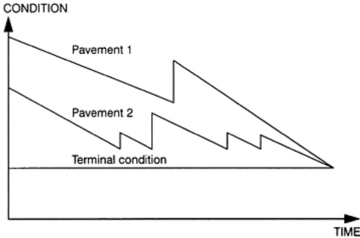
**Figure 16.1** Deterioration as function of time.
