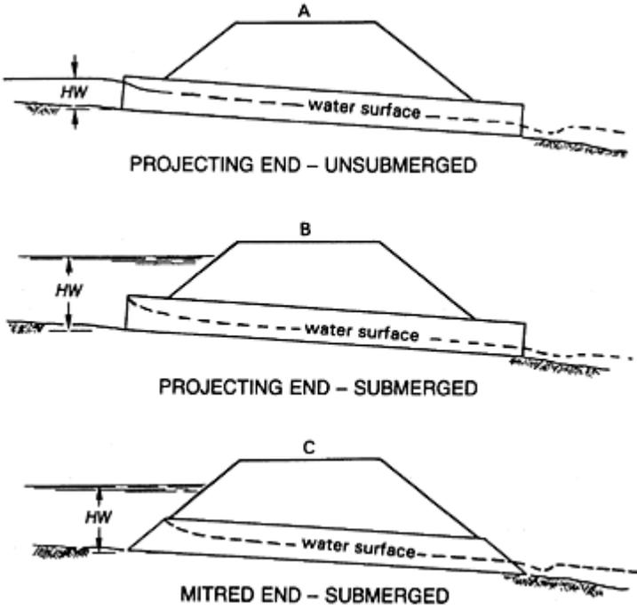
**Figure 11.6** Inlet control (Transportation Research Board, ref. 3).
