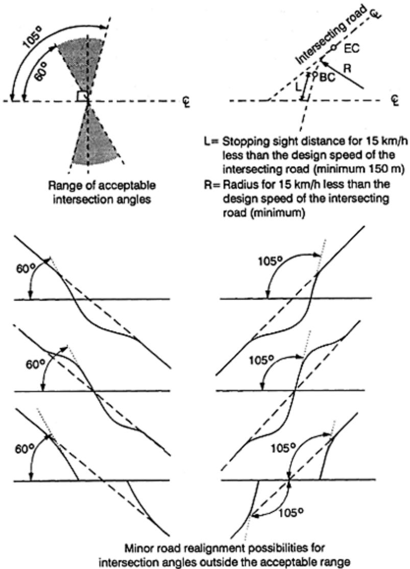
**Figure 8.6** Alignment of intersecting roads (ref. 4).
