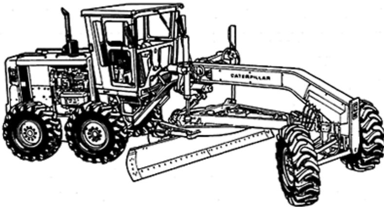
Figure 14.3 Motor grader.
